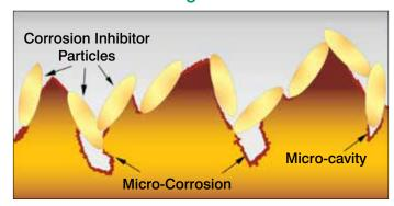
Traditional coatings can not protect the micro-cavities due to the relative large size of corrosion inhibitor particles such as nitrate, aluminum, zinc, and so on.
