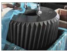
Courtesy Thomas Simone Company Products: VpCI®-126, 369D Paper Mill Gear coated in 369D and wrapped in VpCI®-126 Blue. Location: Ohio, USA
